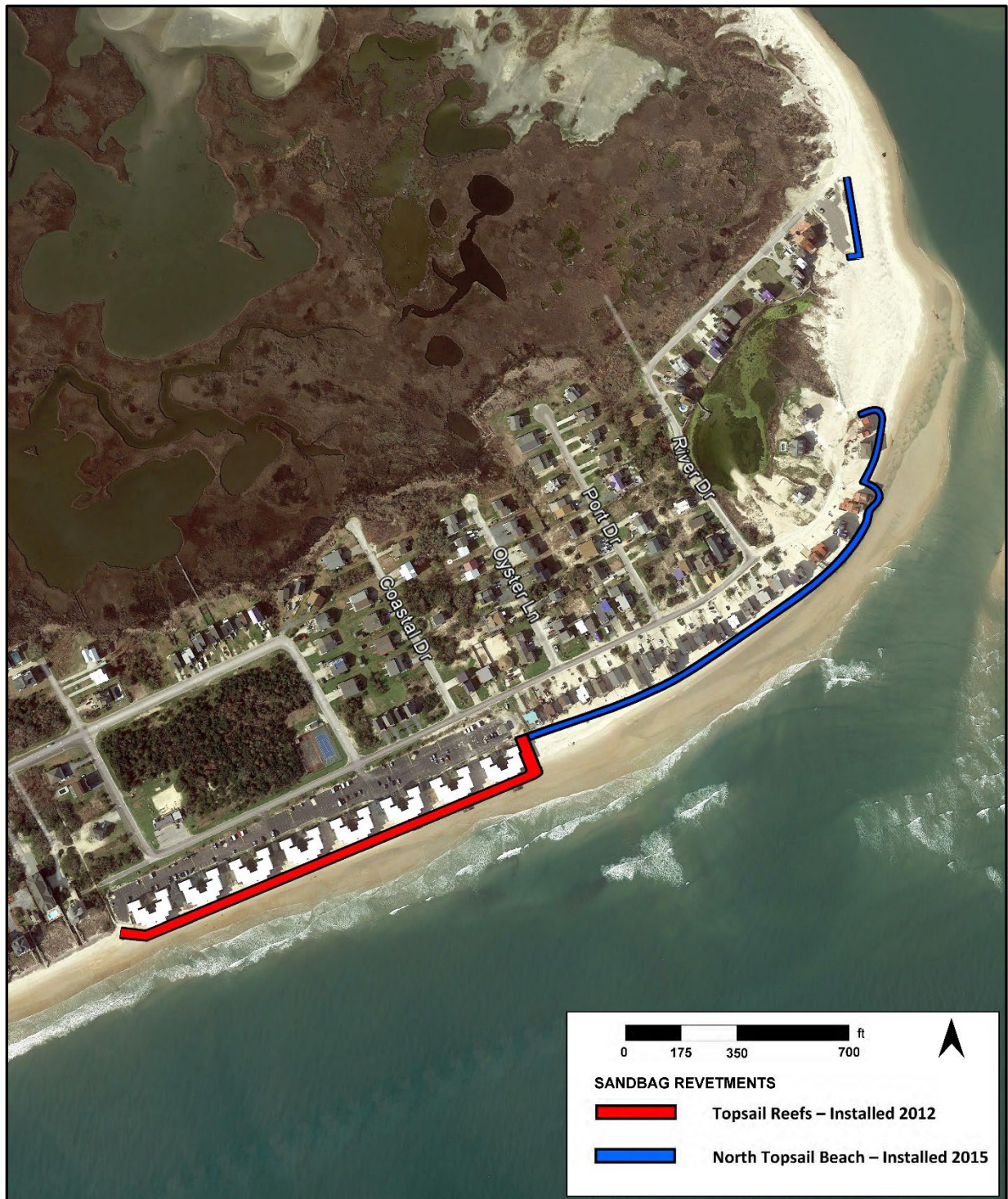
Figure 3-4. North Topsail Beach existing sandbag revetments
