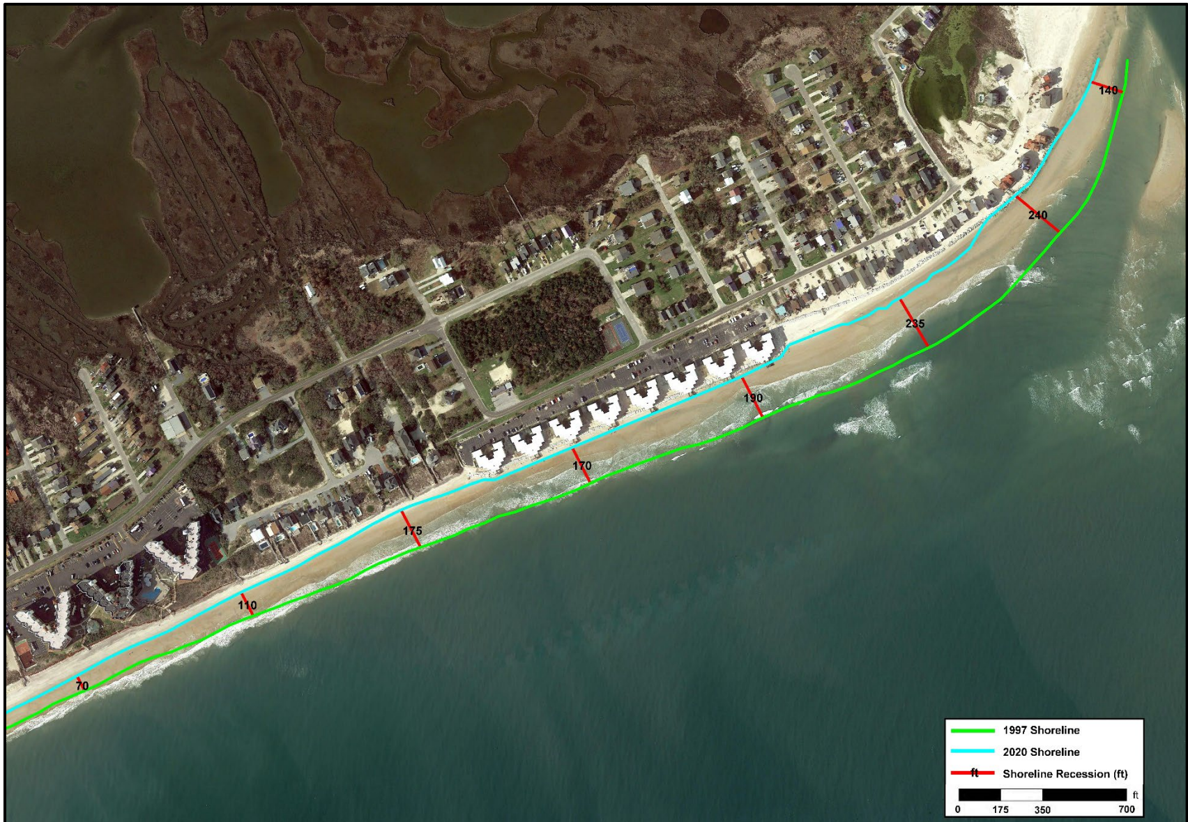
Figure 2-1. North End shoreline recession (ft) 1997 to 2020 (Shoreline Data Source: NCD CM 2022)
