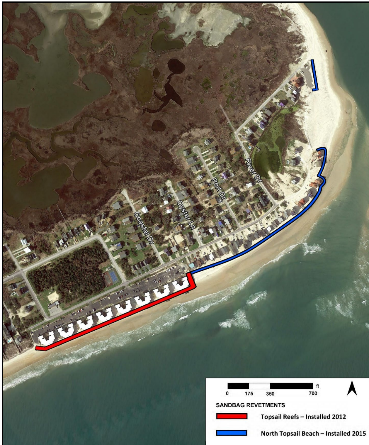
Figure 2-2. Existing sandbag revetments along north end shoreline
