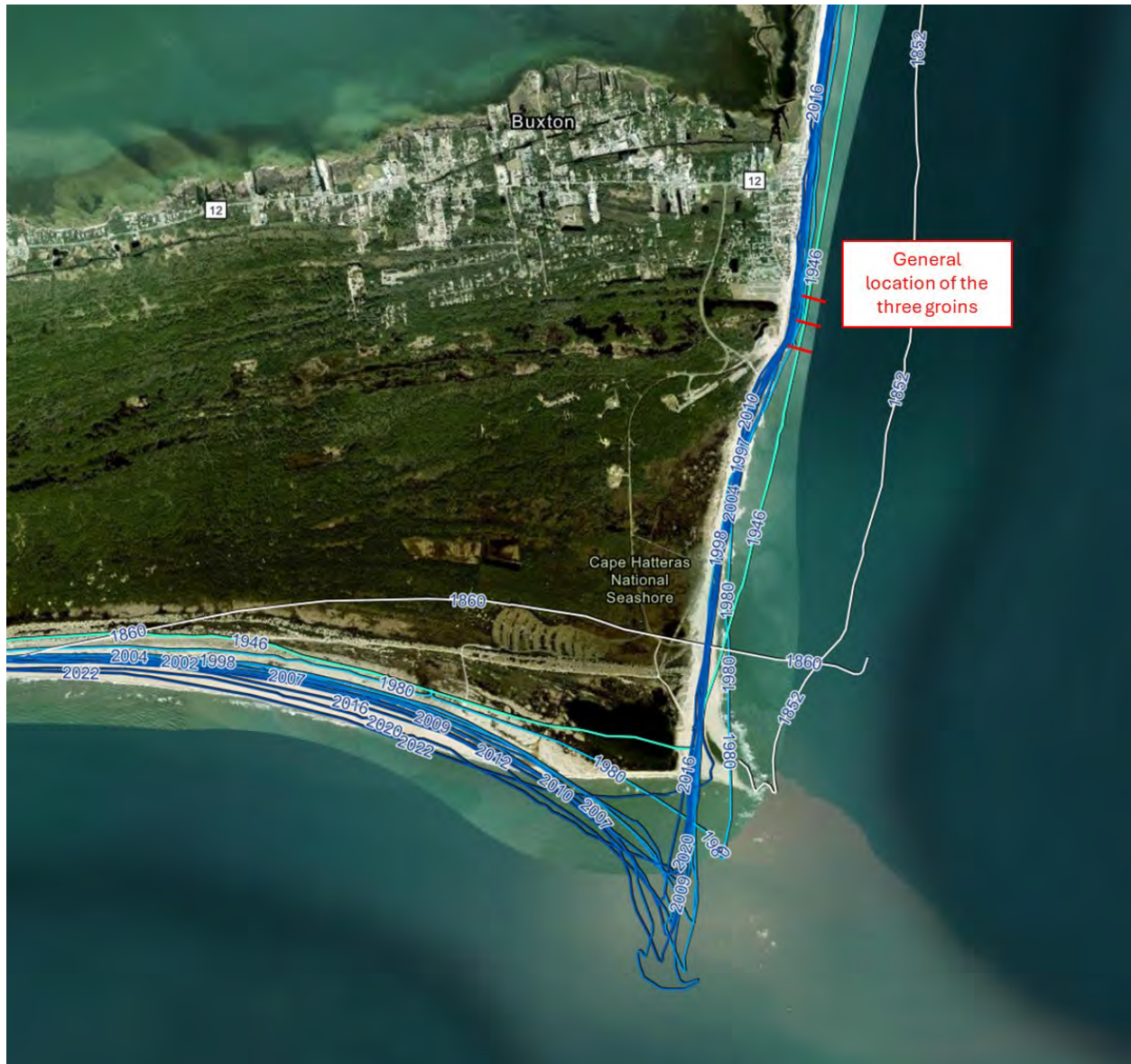
Figure 5. Generalized location of three shore-perpendicular rock and steel groins constructed by the U.S. Navy between 1969 and 1970 to protect former military infrastructure near the Cape Hatteras Lighthouse, NC. Shoreline positions from the NCDCM database are overlaid on 2024 aerial imagery. The groins are not depicted to scale and are commonly referred to as the 1st, 2nd, and 3rd “jetty,” progressing from south to north.
