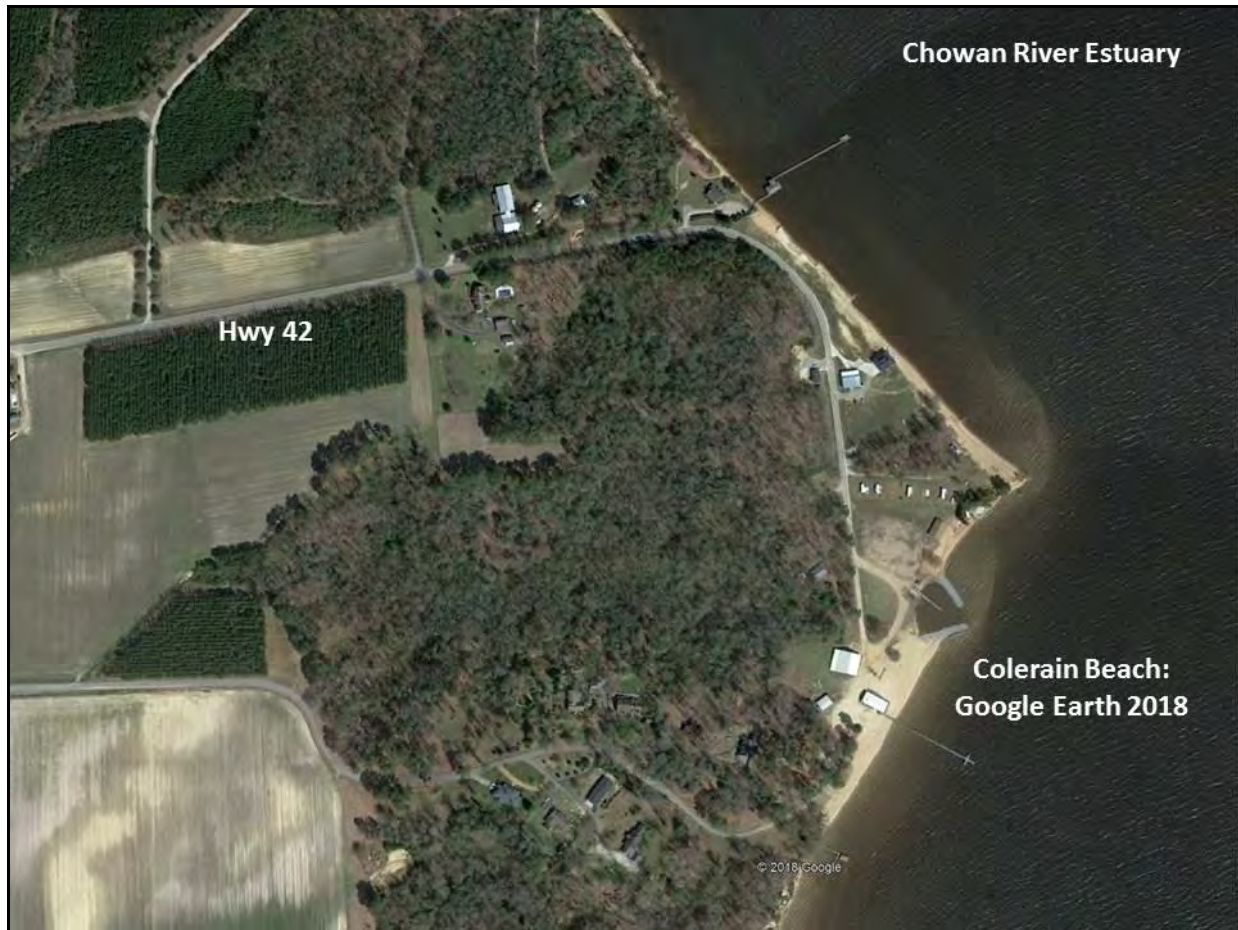
FIGURE 55. A Google Earth (2018) image shows Cape Colerain and its private beach at the east end of NC Highway 42. Notice the boat ramp that is surrounded by massive rock jetties and how they have trapped sand derived from the eroding bluffs to the immediate south of this image.
