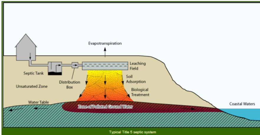
**Figure 4:** Schematic depicting septic system structure and processes as they relate to the surrounding environment (Smart Growth).
