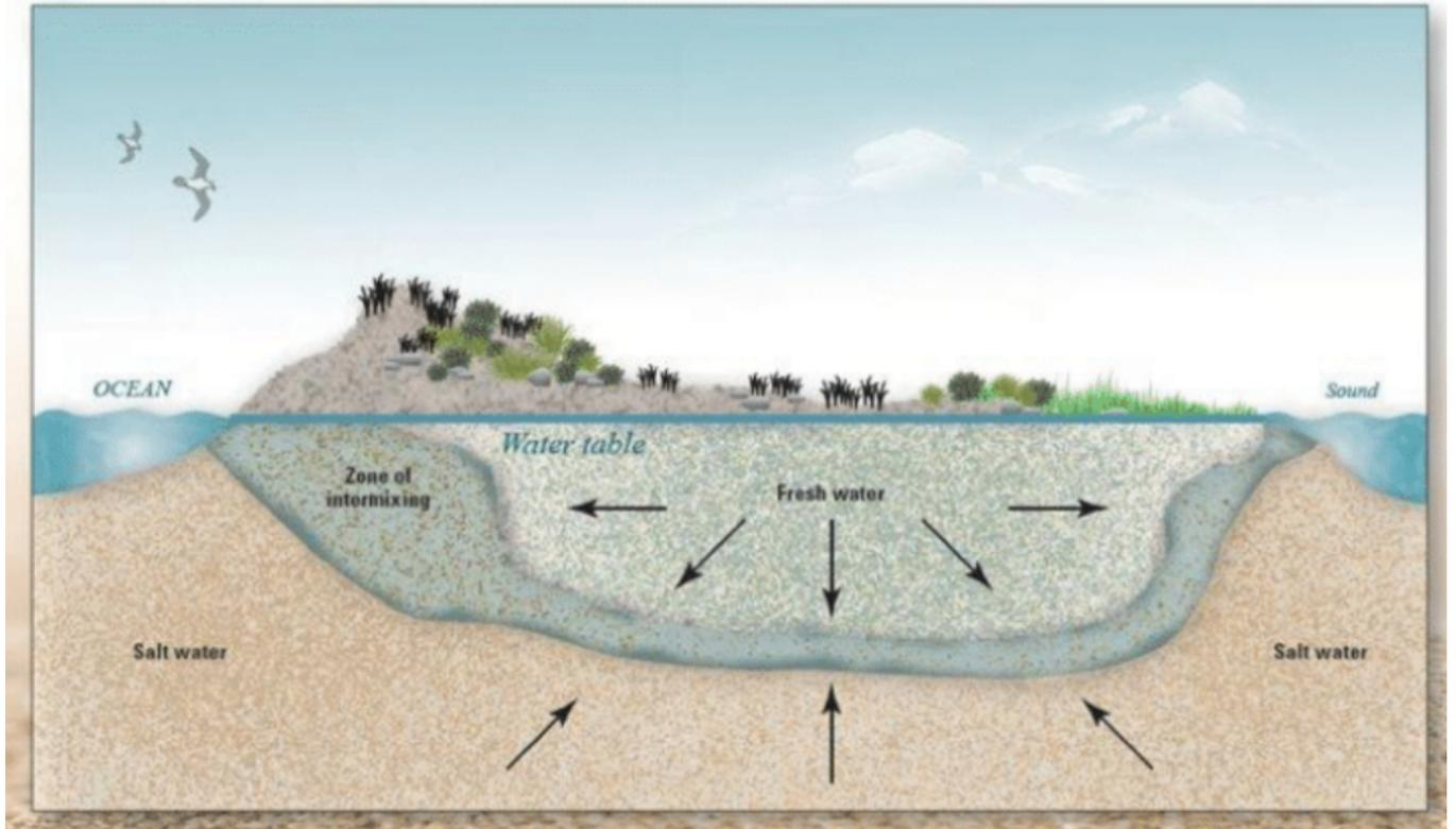
**Figure 2:** Water movement through a barrier island system (reproduced from Dolan, 2016).
